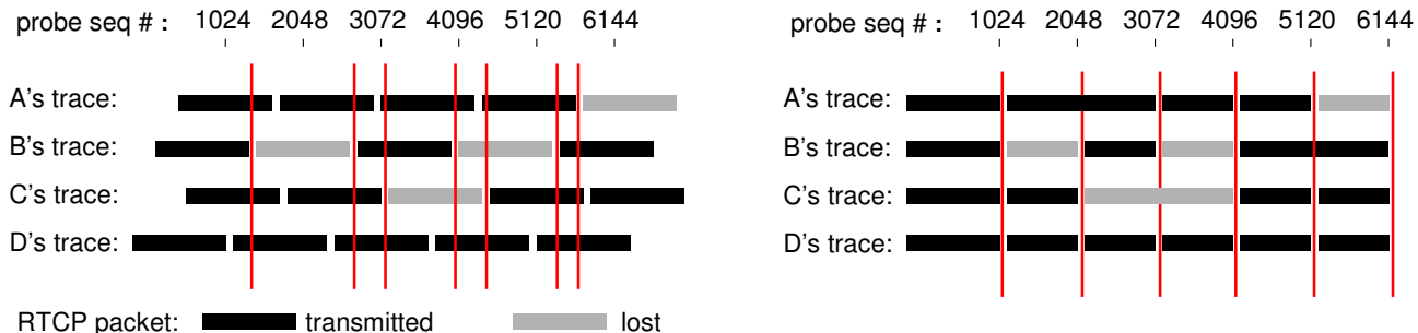
Fig. 3. ALIGNMENT. Without alignment (left), sequence number boundaries of RTCP packets are not coordinated amongst receivers, and hence RTCP packet loss gives rise to complex patterns of overlap (as delineated by vertical lines). Alignment of packet boundaries (right) promotes overlap in the presence of RTCP loss.
