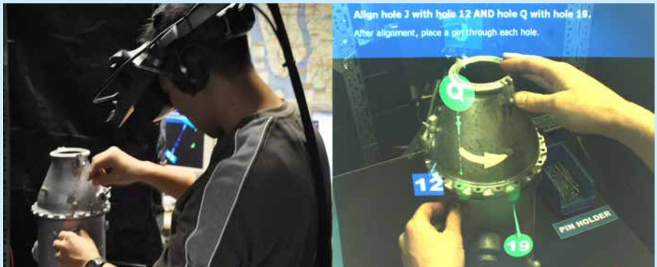
Experimental augmented reality assistance for an aircraft engine assembly task. (Left) Head-tracked optical see-through head-worn display overlays graphics on the user's view of components to be assembled. (Right) View through the head-worn display shows dynamic 3D arrows and labels that provide assistance in spatially aligning components. [Steven Henderson and Steven Feiner, Columbia University]
