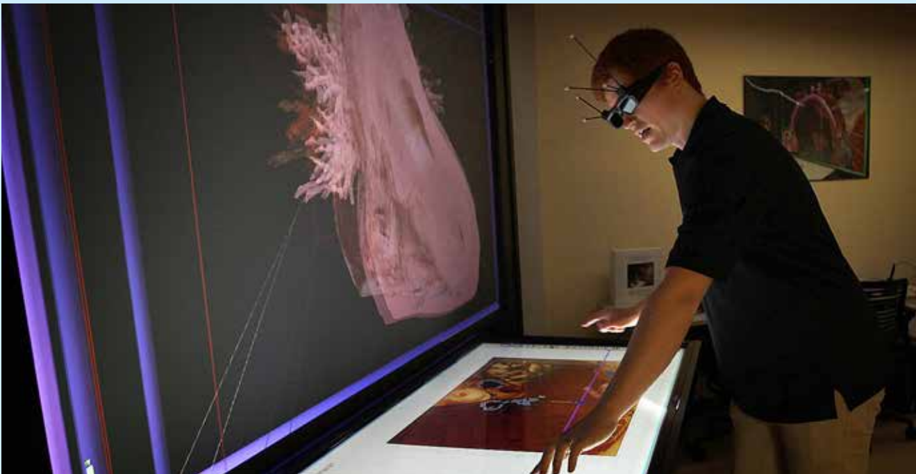
Using fingers, the user is able to virtually enlarge, rotate and dissect images of the heart, veins, arteries and tissue on a massive TV screen projected in three dimensions. The head tracking equipment changes the camera view of the heart based on the user's head movements. [University of Minnesota Interactive Visualization Lab]
